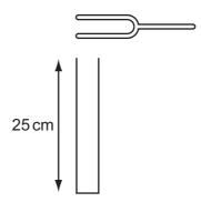
A stationary wave is set up in the tube with the same frequency as the tuning fork. The lower end of the tube is sealed. This is the minimum length of tube with the lower end sealed that creates a stationary wave.
