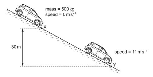
What is the energy dissipated by frictional forces when the car moves from X to Y?
